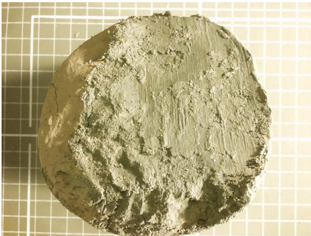
Figure 8.10 View on fault plane in core segment 3 at approx. 912.8 m MD. Fault plane dips towards upper side of photograph. Note slip lines on fault plane.
